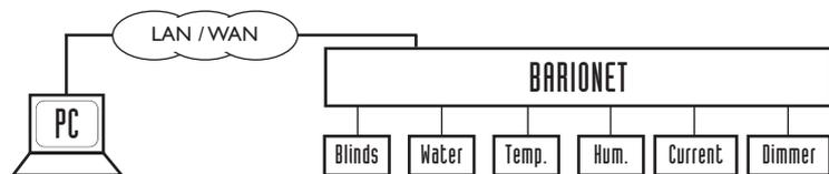
The Barionet comes with standard software featuring fully documented interfaces supporting a variety of different communication methods. UDP and TCP as well as higher level protocols (CGI, XML SOAP) can be selected and SNMP support with a private MIB is available on request.
